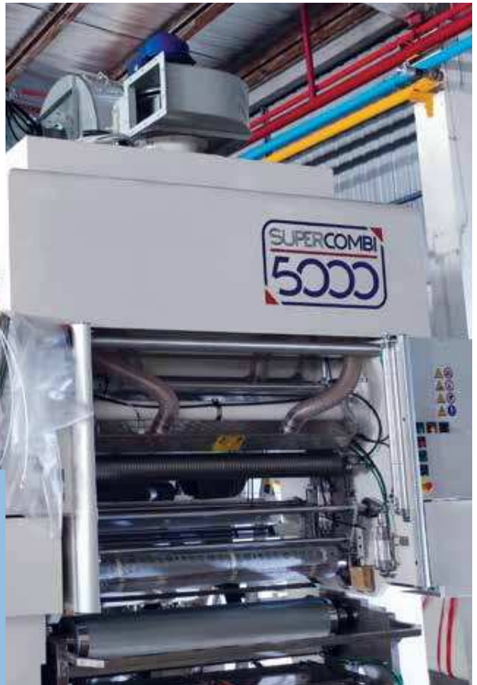
First unit of super combi dry and solventless laminating line.
