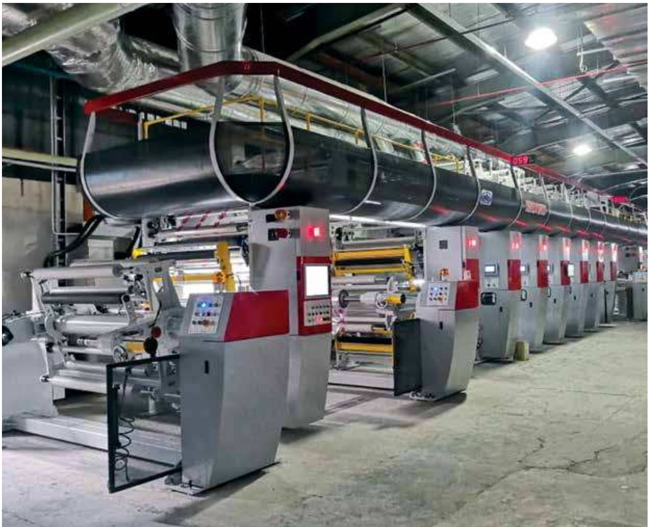
First unit of 6-colour tandem gravure printing line.
